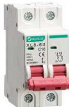
XL8 AC MCB is applicable to a line of AC50/60Hz, 230/400V in single pole, 400V in double, three, four poles for protecting overload and short circuit, and rated current up to 63A. It can also be used for infrequent line conversion under the normal condition. The breaker is applicable to lighting distribution system in industrial enterprise, commercially district, high-rise building and dwelling house. It conforms with the standards of IEC60898 -1.
